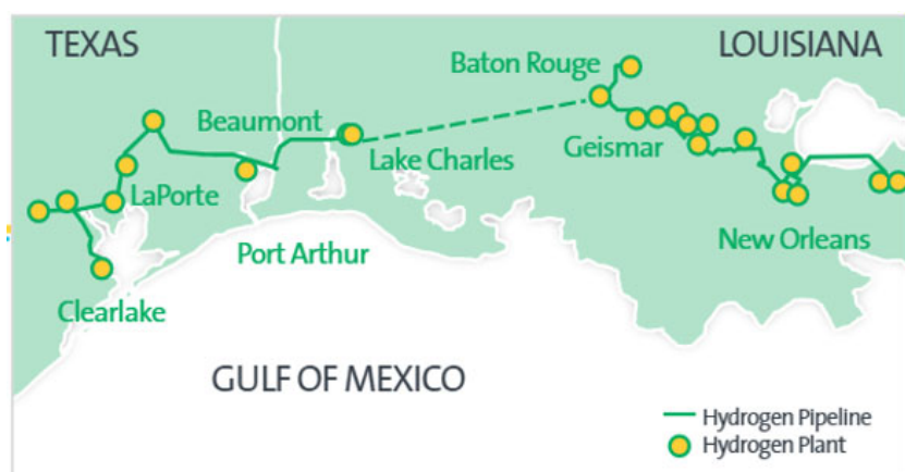
Exhibit 3-4. Example of current hydrogen infrastructure in U.S. Gulf Coast
